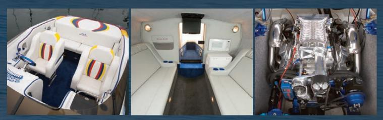
From left: Well-padded gunwales and marine-grade carpet covered the cockpit, which consisted of two manual dropout bolsters and a deep, four-person rear bench. The Water Rod 300's cabin included a bunch of amenities, from a 15-inch, flip-down screen and DVD/CD/MP3 player to a GE microwave oven and recessed cooler. An 800-hp, supercharged, electronically fuel-injected engine from Teague Custom Marine got the V-bottom up to a top speed of 85.8 mph at 5,500 rpm.
