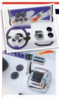
From above: At the helm, the builder installed Mercury SmartCraft gauges in the dash, along with a grab handle for the observer. A chrome electronic throttle and shifter also was included.
