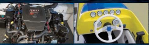
From left: Accompanied with a Bravo One drive, the 300-hp MerCruiser 350 Mag MPI powered the Caliber 1 boat to 63.2 mph at 4,950 rpm. The boat had Faria gauges and a Mercury throttle and shifter.
