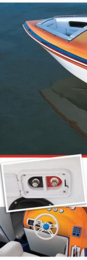
From above: B&H Performance included this remote battery access under the rear bench to charge the battery or provide a jump-start. The helm was completely color-coordinated.
