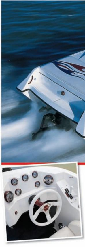
Above: The 27 Sabre's helm featured Beede gauges with color-matched bezels, a non-tilt steering wheel and a Mercury Racing throttle and shifter.
