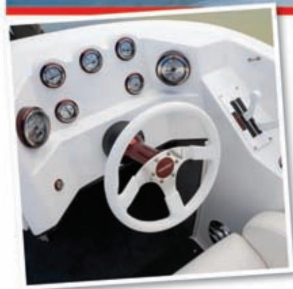
Above: The 27 Sabre's helm featured Beede gauges with color-matched bezels, a non-tilt steering wheel and a Mercury Racing throttle and shifter.
