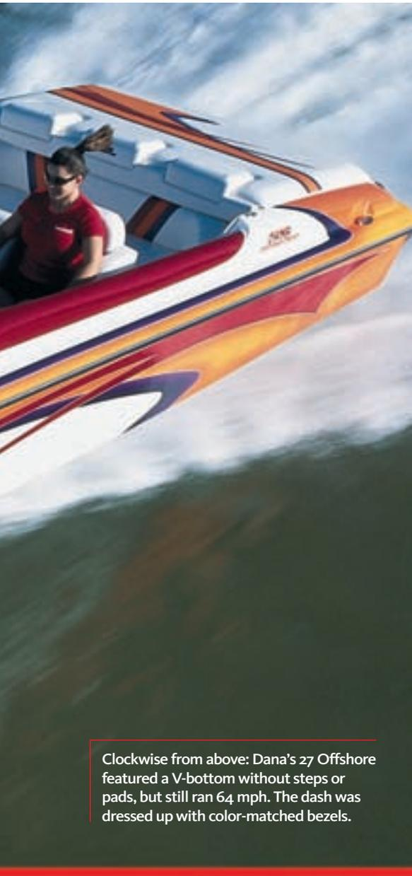
Clockwise from above: Dana's 27 Offshore featured a V-bottom without steps or pads, but still ran 64 mph. The dash was dressed up with color-matched bezels.
